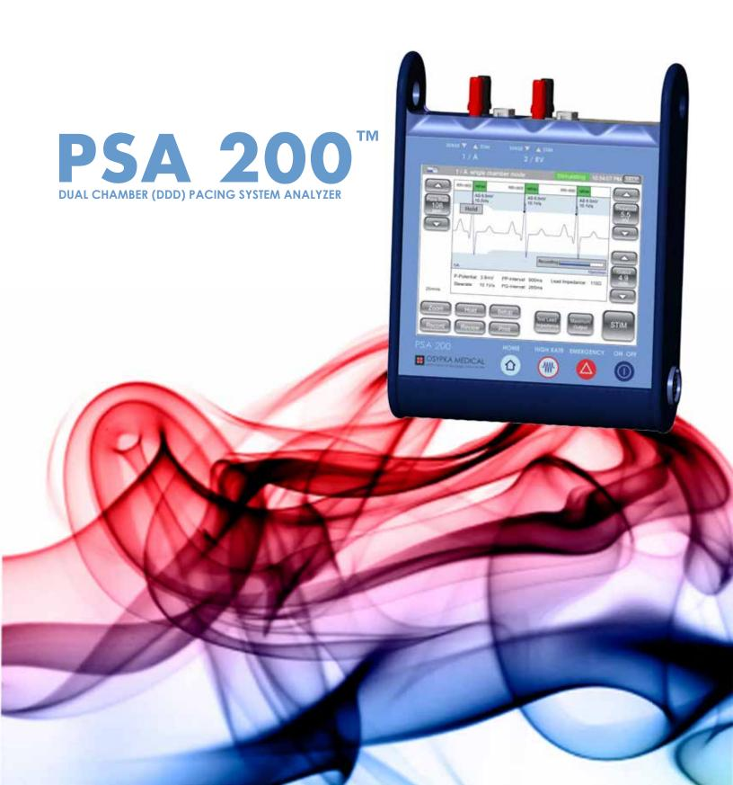
The **PSA 200™** is a standalone, handheld, dual-chamber pacing system analyzer. The system can determine the pacing threshold, commanded or continuous lead impedance, and sensing threshold for each its channels; or resemble a dual-chamber pacemaker in the DDD mode. A user friendly and intuitive touch-screen interface employs only those functions and measurements which are relevant to the specific applications, reducing clutter and confusion.
